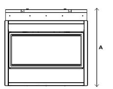
\*Finishing flange depth (The finishing flange defines the perimeter of the fireplace opening). Framing or finishing materials must NEVER encroach inside the finishing flange.
